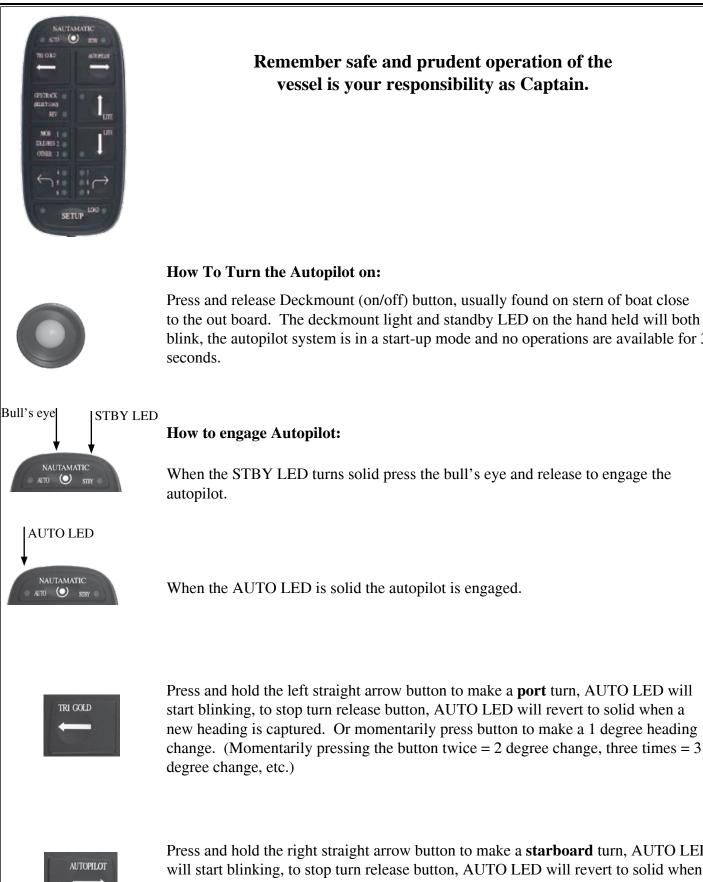
Press and hold the right straight arrow button to make a starboard turn, AUTO LED will start blinking, to stop turn release button, AUTO LED will revert to solid when a new heading is captured. Or momentarily press button to make a 1 degree heading change. (Momentarily pressing the button twice = 2 degree change, three times = 3degree change, etc.)
